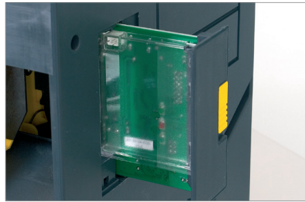
Board easily extractible from the outside
